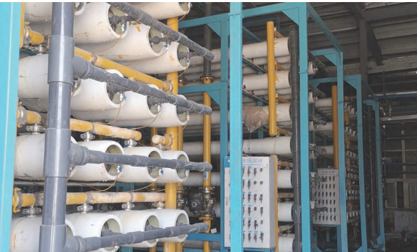
Zero discharge system of electroplating sewage in a metal ecological park in China
